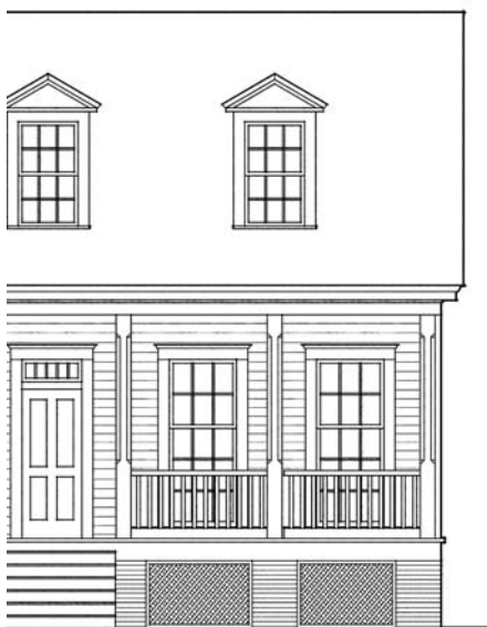
Single-story Porch Partial Elevation
